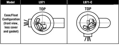
NOTE: Switches shown tripped on falling level.
